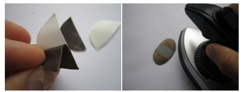
Peel off paper backing from conductive fabric and fuse to neoprene with a medium hot iron
