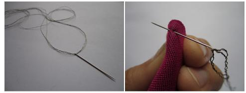
Thread needle with conductive thread and stitch into neoprene
