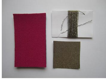
PARTS: neoprene, conductive thread, conductive fabric
