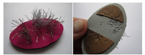
Switch to a non-conductive thread and fill up the rest of the space with non-conductive hairs
