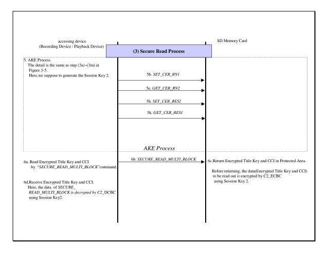
Figure 3-6 – Protocol Flow of "Secure Read Process" from the Protected Area
