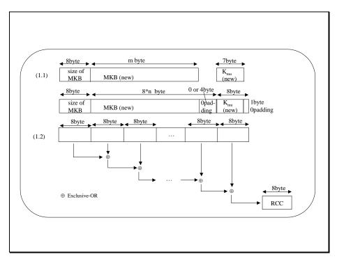
Figure 3-12 – RCC (Redundancy Check Code) Generation Scheme
