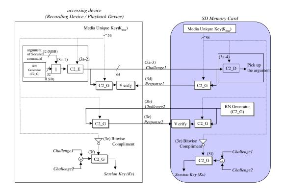
Figure 3-4 – Details of Authentication and Key Exchange (AKE) on SD Memory Card
