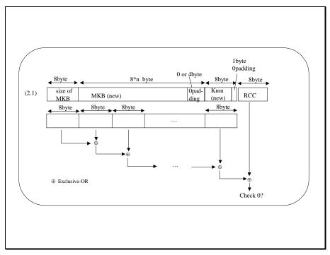
Figure 3-13 – RCC Check Scheme
