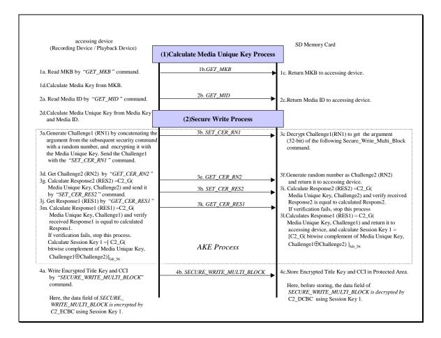
Figure 3-5 – Protocol Flow of "Secure Write Process" to the Protected Area
