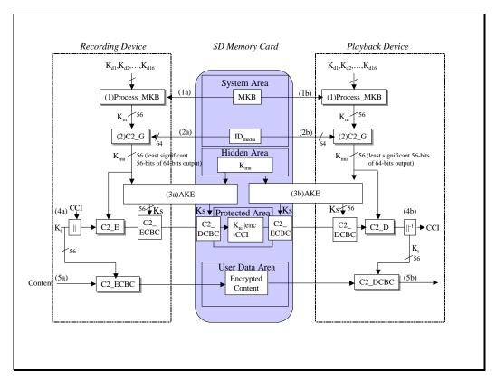
Figure 3-3 – Content Encryption and Decryption on SD Memory Card
