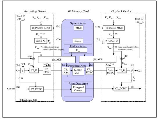
Figure 3-14 - Content Encryption and Decryption on additional ID Binding
