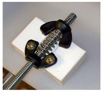
Turn the wing nuts so they put a small amount of tension on the spring. You want them close enough together and compressing the spring just enough to remove any play in the wing nuts, but not so tight that it becomes difficult to turn them on the rod.
