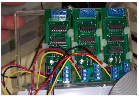
MyDIYCNC Stepper Driver Modules have labels on the board, as shown in the illustration, indicating the purpose of each connection.
