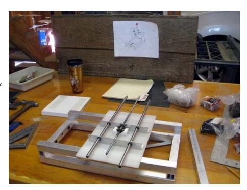
aligned, tested for squareness and then clamped/secured in the precise location <u>before</u> drilling a pilot hole and screwing them together.
