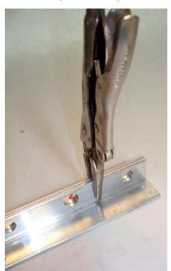
bearing frames to length in pairs. Clamp each pair back to back, as shown in the illustration, ensuring that the pieces are perfectly aligned. Drill the 7/16" holes for the bearings and to clear the threaded rod as shown in the drawings. Mark each pair to keep them together and not mixed up with the other bearing sub frames.
