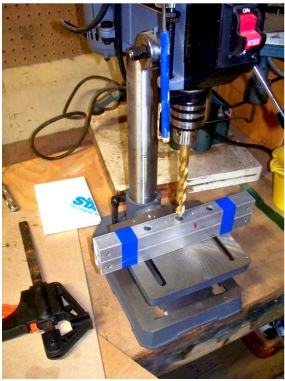
Clamp or tape together rail pairs for drilling to ensure alignment of holes
