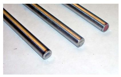
Using a metal file or grinding wheel, chamfer the ends of each cut rod to remove any burrs and to bevel off the shoulder of the cut. This will make it easier to locate each rod in its hole/pocket/grommet without causing damage as the rod is inserted.
