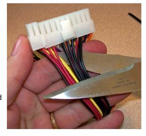
illustration). Fold all the other unnecessary (non black, red or yellow) wires careful back into the power supply case. As long as you have a standard ATX PC power supply, there should be sufficient space to do this.
