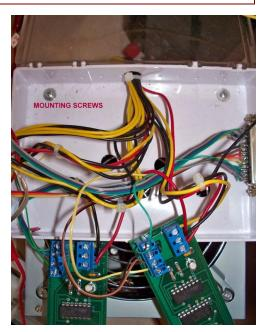
The electronics boards are designed to be mounted in the enclosure using PCB edge standoffs. If using the MyDIYCNC enclosure, the electronics boards are mounted to the lid of the enclosure as shown. This allows for greater access to the boards and wiring. You may choose to mount them otherwise if preferred.
