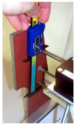
Likewise, the bearing holes in the bearing sub frames must be centered to the exact same dimension as the distance between centers of the rods. The Igus bearings allow for about .01" of tolerance when mounted in 7/16" holes, but precision in mounting the bearings on the
