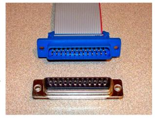
ribbon cable to the electronics, be careful to note the pin number for each strand before connecting to the electronics.
