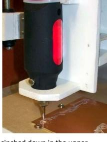
tight and firm fit. Once cinched down in the upper cradle, the spindle should feel solidly fixed in position without any play or movement between the spindle and the Z carriage.
